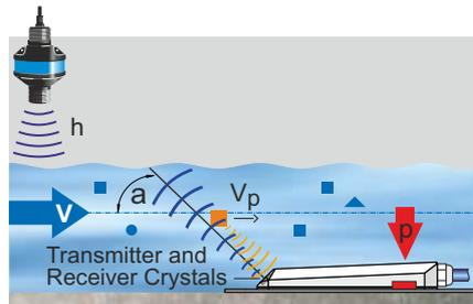
$p$  = Level measurement with pressure (combi sensor)
