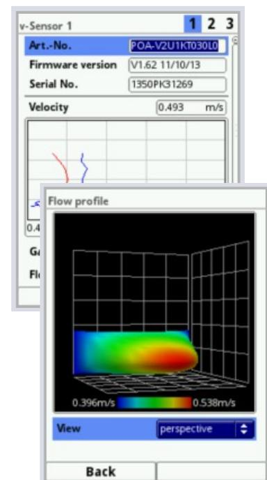
The NivuFlow 750/700 uses up to 9 x 16 gates for flow measurement. A flow profile can be directly indicated on the display.
