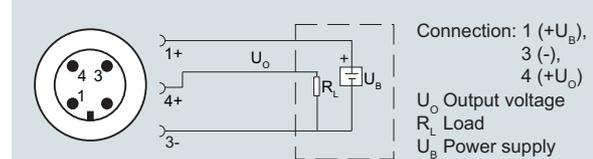
Connection with voltage output, ratiometric output and device plug M12x1
