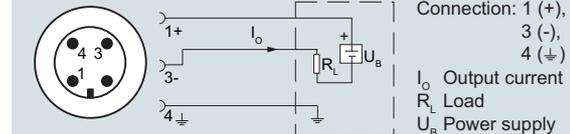
Connection with current output and device plug M12x1 (Ex)
