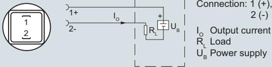
Connection with current output and connector per EN 175301
