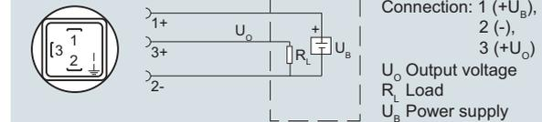
Connection with voltage output, ratiometric output and plug according to EN 175301
