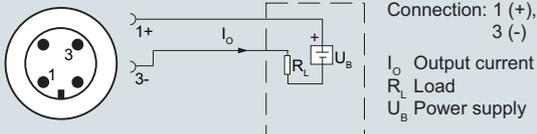
Connection with current output and device plug M12x1
