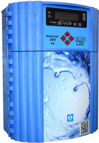
The **Testomat 2000® Fe** process photometer is an online analytical instrument for monitoring the dissolved iron (II) + (III) content in the range from 0 to 1.0 mg/l (ppm) using the photometric analysis principle.
