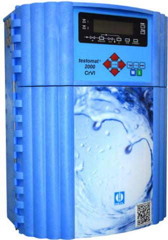
The **Testomat 2000® CrVI** process photometer is an online analytical measuring instrument for monitoring the content of chromate ( $\text{CrO}_4^{2-}$ ) or chromium VI (CrVI). The instrument works with a photometric analysis principle based on DIN 38405. Two device variants are available for the realization of the most diverse measurement requirements.
